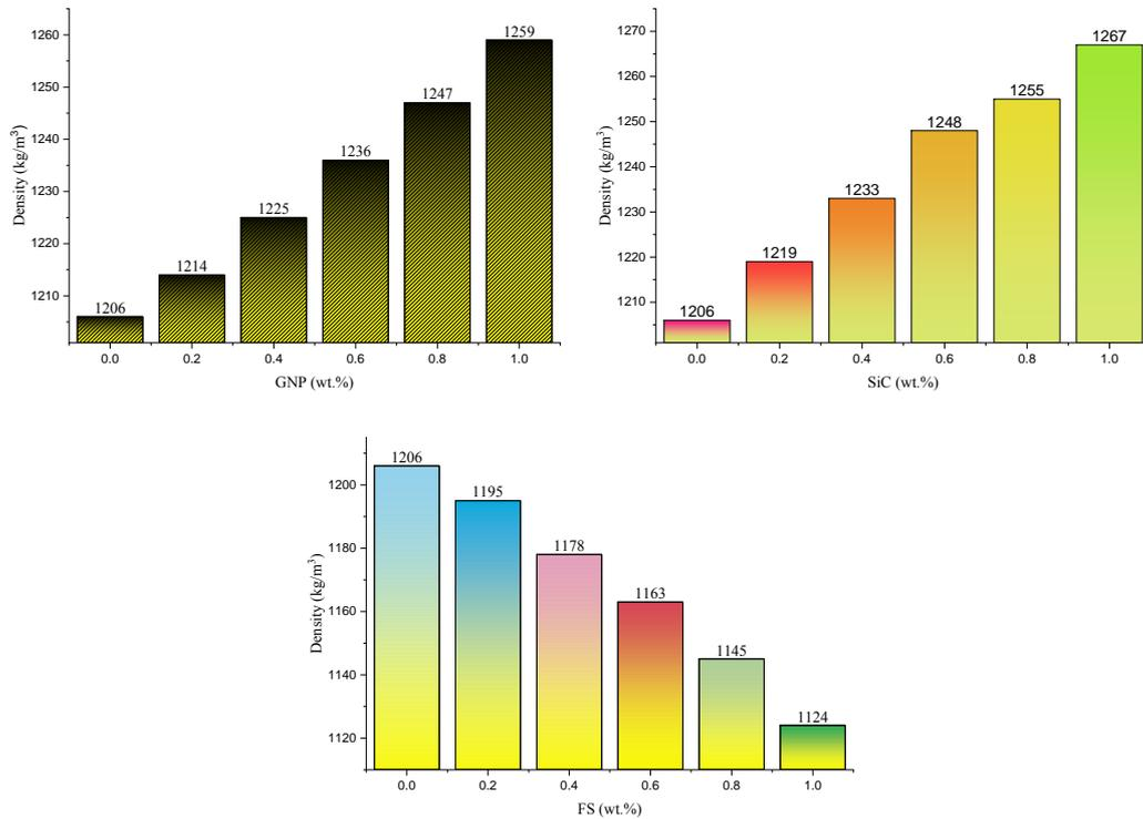
**Figure 4.** Effect of GNP, SiC, and FS reinforcement on the density of the polyester nanocomposite
