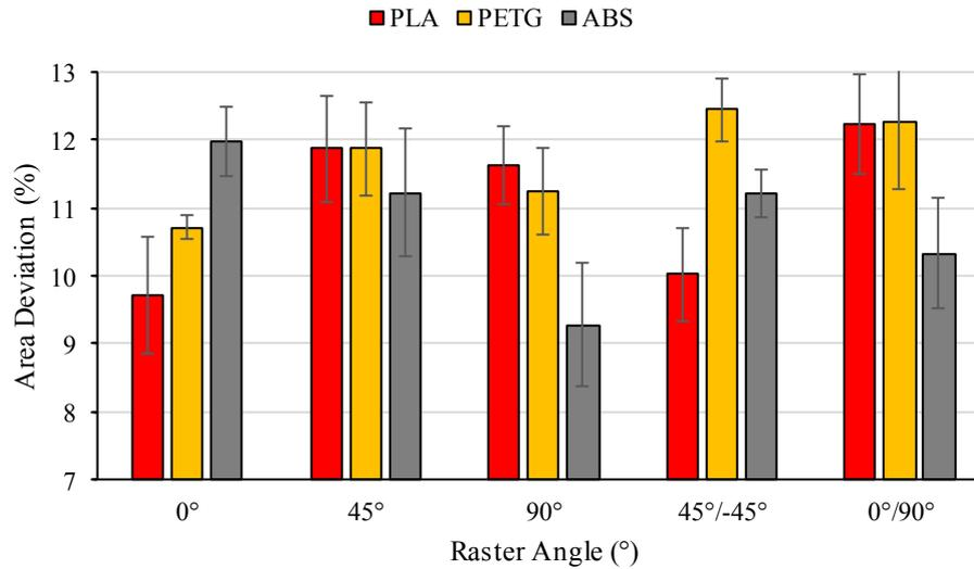
**Figure 7.** Cross-section area deviation (%) with raster angle (°).
