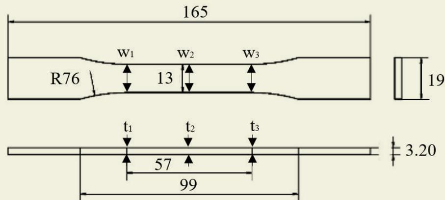
**Figure 1.** The CAD geometry of the printed samples with the positions of the dimensional accuracy measurements ( $w_1$ ,  $w_2$ ,  $w_3$ -width measurements;  $t_1$ ,  $t_2$ ,  $t_3$ -thickness measurements)
