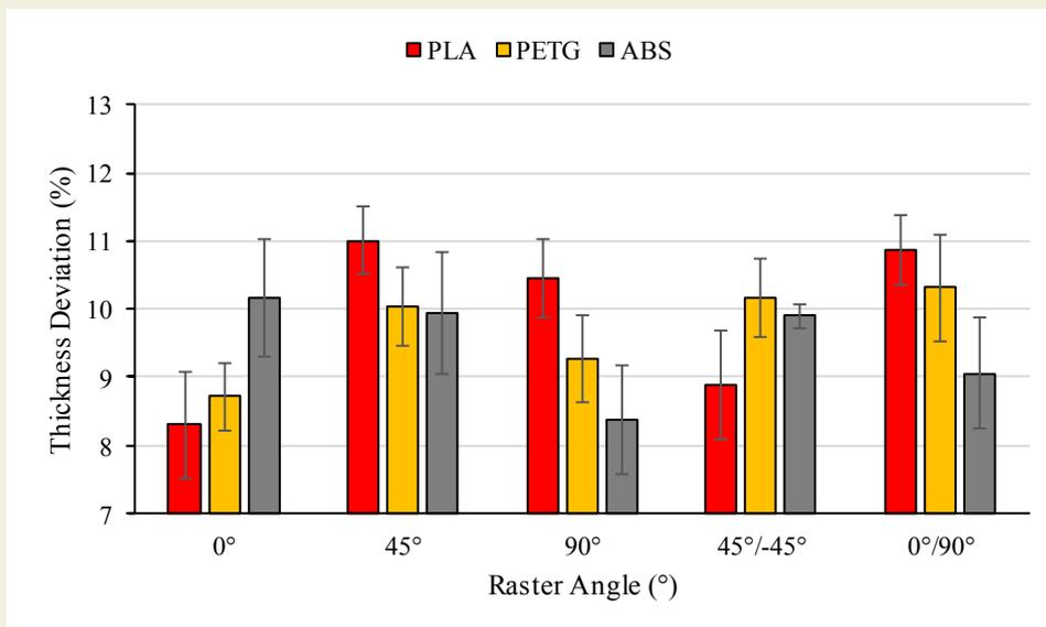
Figure 5. Thickness deviation (%) with raster angle (°).
