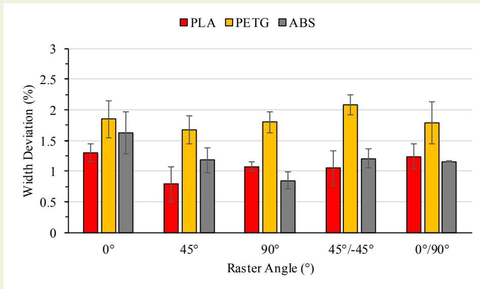
Figure 4. Width deviation (%) with raster angle (°).
