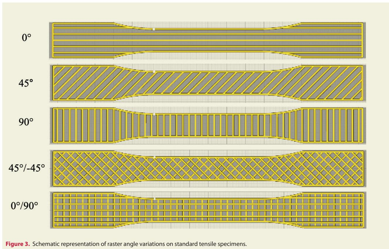
**Figure 3.** Schematic representation of raster angle variations on standard tensile specimens.
