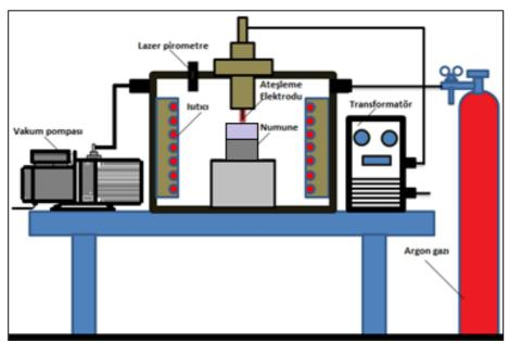
Figure 2: The scheme of ignition unit[13]
